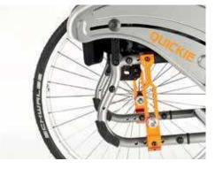
**Seat height adjustable in seven positions** With a camber from 0° to 4° and four centre of gravity positions (from the very active 8.3cm to the more steady 2.3cm).
