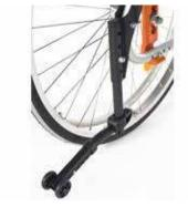
**NEW Lightweight anti-tip** for optimal driving performance with 480g weight reduction.
