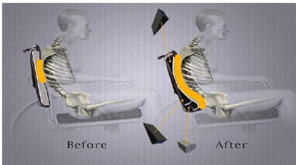
In the 'before' picture a J3 back shallow contour, upper thoracic is attached to the backposts. When the user sits against the back, his support is concentrated in a small area, resulting in peak pressure which may result in compromised skin integrity and discomfort over time. Postural stability is also compromised.
