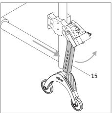
• Once the wheels are fitted, you can return the anti-tippers to their starting position. To do this, push the wheelchair forwards and at the same time push back the holding rod [15] using your foot.
