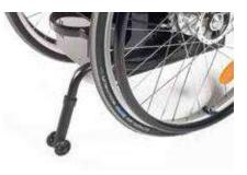
Anti-tip Increased stability without adding too much weight. The anti-tip can be flipped up manually.
