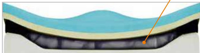
Cross section showing integral fluid insert
